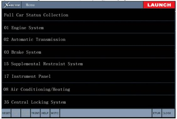
Here lists "Full Car Status Collection" and all systems. Currently, VW/AUDI car models support test for 102 systems. Under this menu, user can directly select the system to be tested. After selecting the corresponding system, it displays all the functions of this system. Selecting "Full Car Status Collection"
