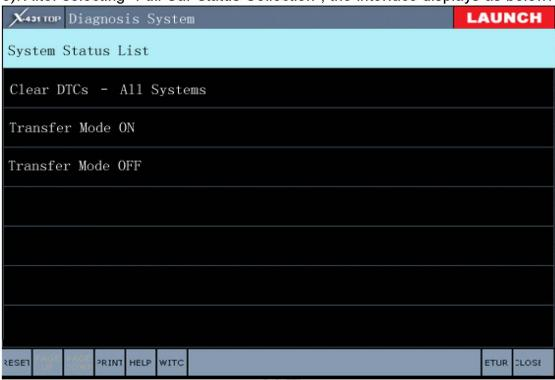
4). When selecting "System Status List", it will list equipped systems and the status of each system. Interface as below:
