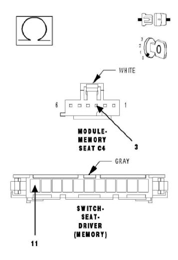
5). CHECK THE (P239) DRIVER SEAT REAR VERTICAL/HORIZONTAL SWITCH MUX WIRE RESISTANCE
