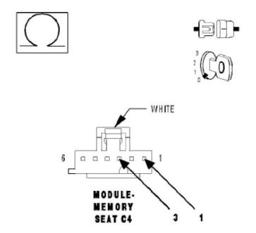
4). CHECK THE (P339) DRIVER SEAT FRONT VERTICAL/RECLINER SWITCH MUX WIRE RESISTANCE
