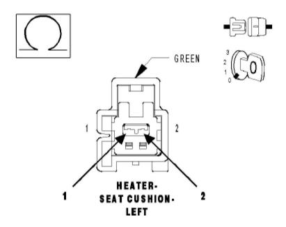
3). CHECK THE LEFT SEAT BACK HEATER RESISTANCE Disconnect the Left Seat Back Heater 2 – way connector. NOTE: Check connectors - Clean and repair as necessary. Check the resistance of the seat back heater element by measuring between the (P187) Left Seat Heater B(+) Driver and the Ground circuit at the connector.
