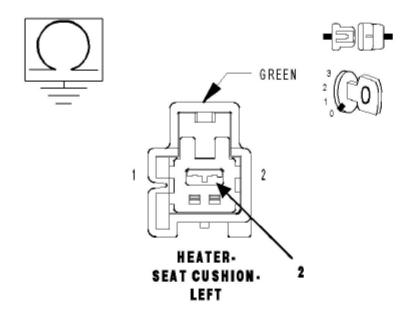
5). Check the (P187) Left Seat Heater B(+) Driver circuit for an open. Disconnect the Heated Seat Module connector.
