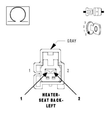
4). CHECK THE LEFT SEAT HEATER GROUND CIRCUIT RESISTANCE Measure the resistance of the Ground circuit at the Left Seat Heater Cushion 2 – way connector.
