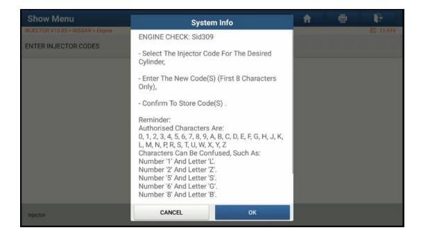
4. If we changed the injector of cylinder 1, we need to select "CYL1".
