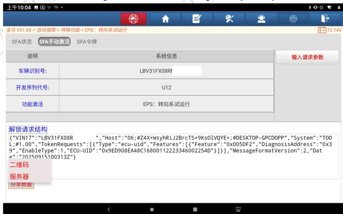
10.1 Start connecting to the server to upload data. After the data is uploaded successfully, a QR code will be displayed. Use WeChat to scan the QR code to open the website.
