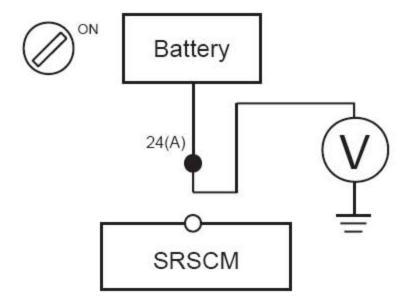
C) Is the measured voltage within specification?
