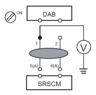
D) Is the measured voltage within specification?
