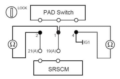
C) Is the measured resistance within specification?
