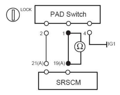
C) Is the measured resistance within specification?
