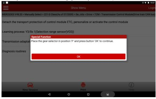
10). After clicking OK and prompted success, it shows "Place the gear selector in position R". After engaged in position R, click OK button:
