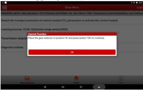
12). After clicking OK and prompted success, it shows "Place the gear selector in position D". After engaged in position D, click OK button:
