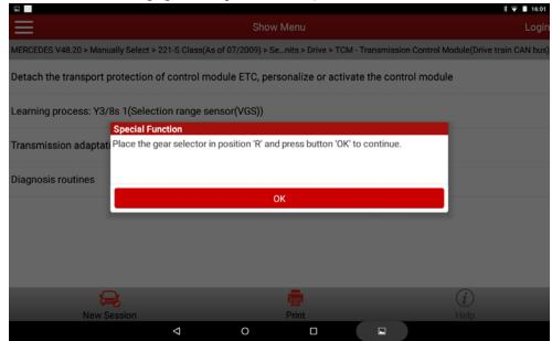
11). After clicking OK and prompted success, it shows "Place the gear selector in position N". After engaged in position N, click OK button:
