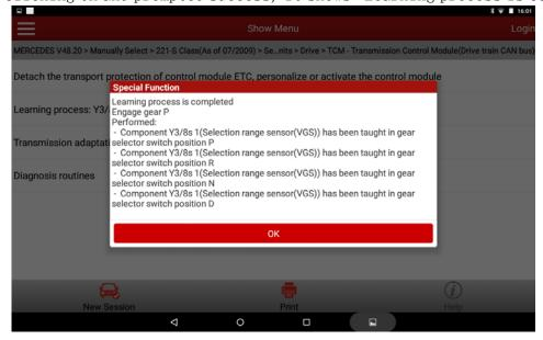
14). After gearbox self-learning succeeded, turn the key off, and exit from the software. Start the engine, idle works normally. Test on road, gears can be shifted normally and vehicle starts normally, which indicate the gearbox self-learning succeeded.
