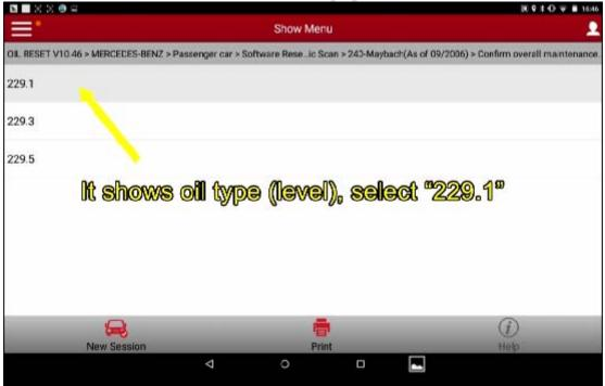
10). Select any type (level), it will display "Oil reset completed". Click OK to complete.
