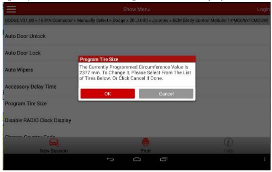
12). Select the correct menu according to the replaced tire.
