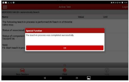
14). Click OK. After about 10s, the system returns to the menu page. Turn off the ignition switch. The operation is complete.
