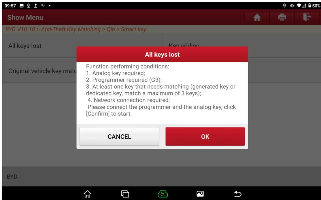
6. Connect the relevant devices and vehicle according to the connection sketch map, and then click [OK] (shown in the following picture)
