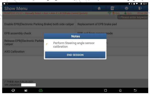
6. "BCS – SAS (Steering Angle Sensor) calibration" is executed successfully. (See the following figure.)
