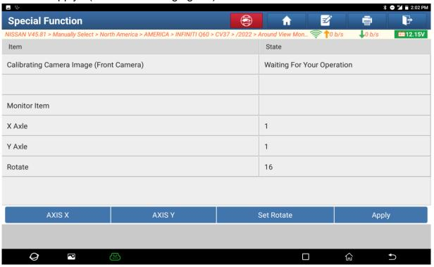
8. After clicking "Apply", observe whether the image in the central control screen is correct. If not, re-enter the valuesof "X Axle" and "Y Axle" and click "Apply" to adjust. After the adjustment is correct, click OK to proceed. (See the following figure.)
