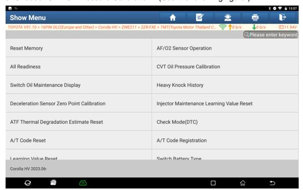
4. Recalibrate the CVT oil pressure after replacing related parts. Click OK. (See the following figure.)
