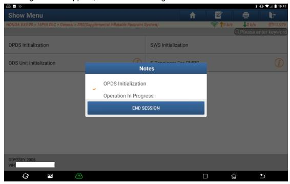
6. After the initialization is completed, wait for 10 seconds, and then the software will clear the ECU DTCs, as shown in the figure below.
