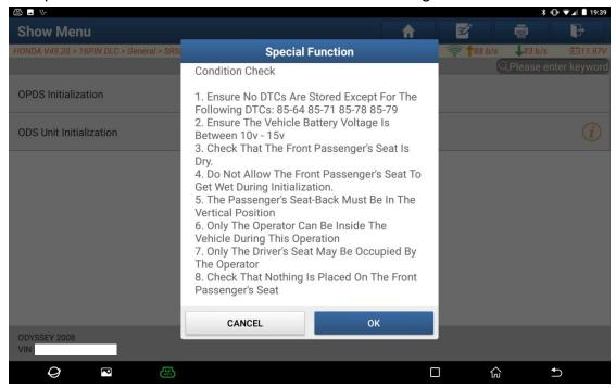
4. Click OK when the conditions are met. According to the prompt information, turn off the ignition switch, wait for 10 seconds, and turn on the ignition switch. Then, wait for another 10 seconds until the figure below is displayed. Click OK to start the initialization operation.
