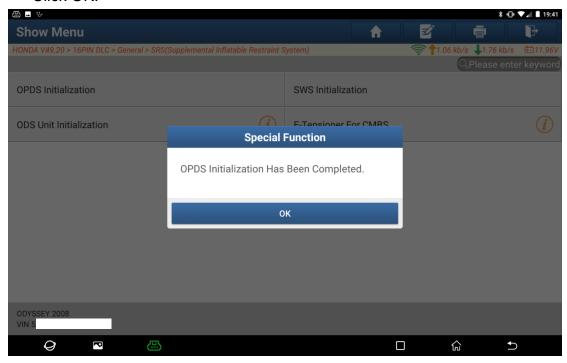
8. Note that it is forbidden to power off during the initialization operation, as shown in the figure below.
