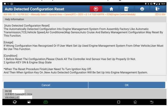
3. Turn on the ignition switch, turn off the engine, and click OK.
