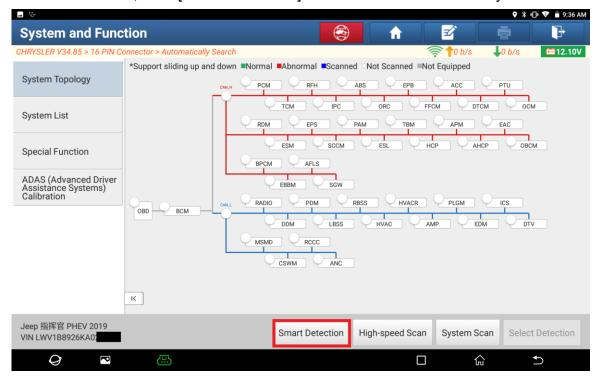
7. Click [BPCM (Battery Pack Control Module)] to access the system.
