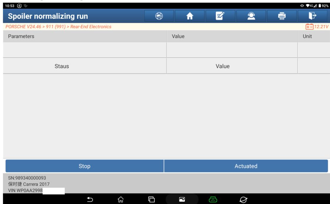
7. Actuation test status is [Function completed], spoiler calibration succeeded;
