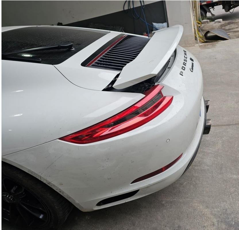
When depressed spoiler panel button, the button light is flickering, but spoiler cannot be stowed
