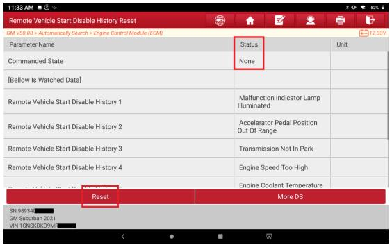
11:33 AM 🖪 🛞 ৬ Remote Vehicle Start Disable History Reset Ħ **Q** 3 Status Unit Parameter Name Commanded State Reset [Bellow Is Watched Data] Remote Vehicle Start Disable History 1 None Remote Vehicle Start Disable History 2 None Remote Vehicle Start Disable History 3 None Remote Vehicle Start Disable History 4 None Remote Vehicle Start Disable History 5 None Reset More DS SN:989340 GM Suburban 2021 VIN 1GNSKDKD9MF
