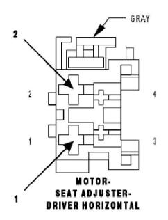
5). CHECK THE (G401) DRIVER SEAT HORIZONTAL POSITION SENSE WIRE FOR AN OPEN
