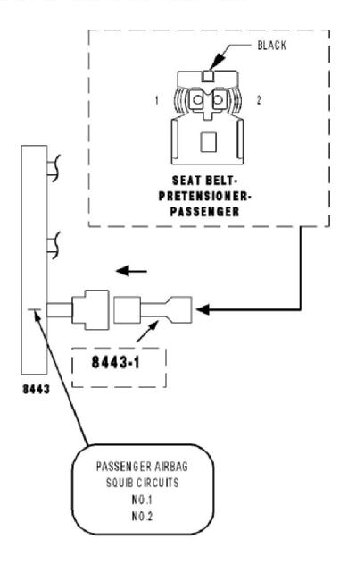
3). CHECK (R56) PASSENGER SEAT BELT TENSIONER LINE 1 CIRCUIT AND (R54) PASSENGER SEAT BELT TENSIONER LINE 2 CIRCUIT FOR A SHORT TO GROUND
