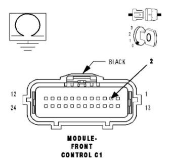
6). (D54) CAN B BUS (-) CIRCUIT FOR A SHORT TO GROUND NOTE: Ensure each CAN B Bus module is disconnected at this time.
