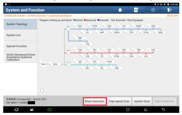
7. Click [ABS (Anti-lock Braking System)] to access the system.
