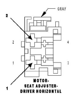
5). CHECK THE (G402) DRIVER SEAT REAR VERTICAL POSITION SENSE WIRE FOR AN OPEN
