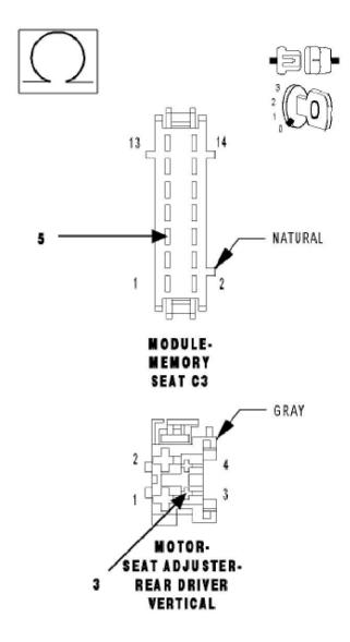
7). CHECK THE (P111) DRIVER SEAT REAR VERTICAL UP DRIVER WIRE FOR AN OPEN
