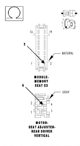
6). CHECK THE (G492) DRIVER SEAT REAR VERTICAL SENSOR GROUND FOR AN OPEN
