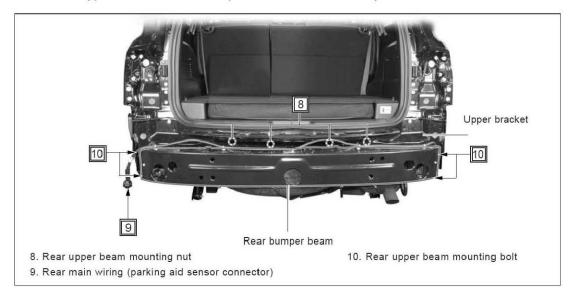
Unscrew four upper beam mounting bolts and remove the upper beam assembly.
