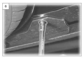
Remove the lower mounting bolts (LH/RH, 12 mm) from the rear bumper.
