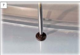
7. Remove five rear mounting scrivets and remove the rear bumper fascia.
