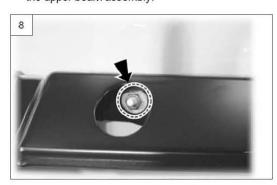
Disconnect the rear main wiring (parking aid sensor) connector and the connector mounting piece on the side of the body.
