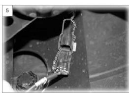
5. Disconnect three parking aid sensor connectors (LH/C/RH).
