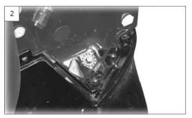
3. Remove the rear wheel house mounting screws.
