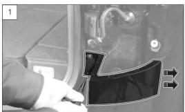
Remove two rear extension cover mounting screws and remove the rear combination extension cover by sliding it.
