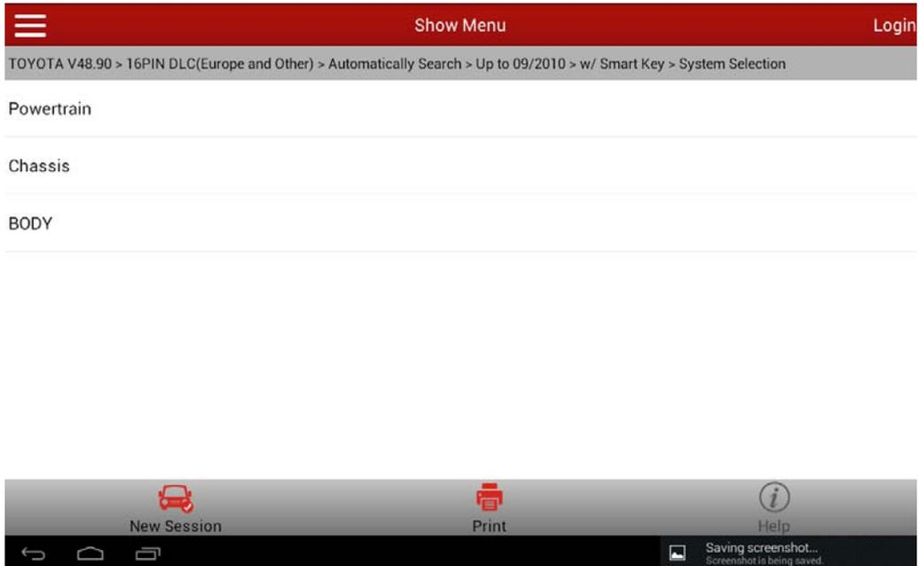
9). Select ABS (Anti-lock Brake System)/VSC (Vehicle Stability Control)/TRC (Traction Control).
