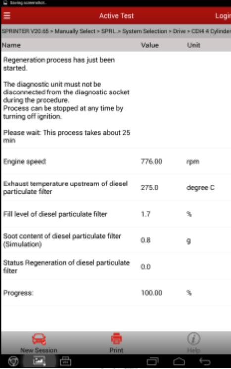
The screenshot shows the 'Active Test' interface for a SPRINTER V20.65. The test is for 'CDM 4 Cylinder'. The interface displays a table of parameters during the DPF regeneration process.
