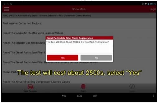
17). After clicking YES, the vehicle enters preparation stage, which lasts several seconds or several minutes. Then the engine speed increases to a constant high speed (approx. 2500rpm). The engine runs about 25 minutes at this high speed before it decreases to idle. After idling for 100 seconds, it prompts you to turn the key to OFF position. Now, the static regeneration is executed successfully.
