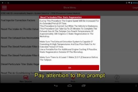
12). After all conditions are satisfied, turn the switch ON, then start engine and monitor the engine coolant temperature, prompted.
