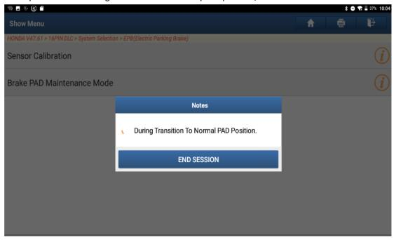
9. The EPB (Electronic Parking Brake) system is switched to the normal brake pad position, the function is completed, click "OK", as shown below:
