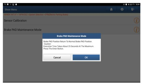
8. In the process of switching to the normal friction plate position, as shown below:
