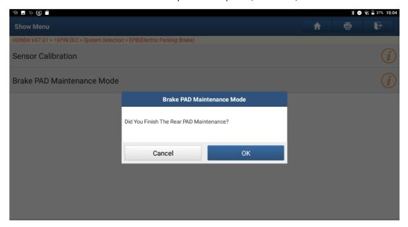
7. Click "OK", the brake pad position returns to the normal brake pad position, as follows Figure:
