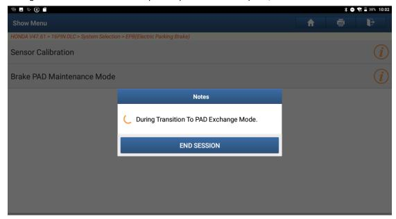
6. After the maintenance of the rear friction plate is completed, click "OK", as shown below:
