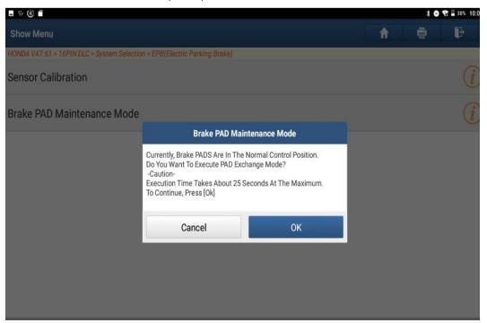
5. During the transition to the friction plate replacement mode point, as shown below:
