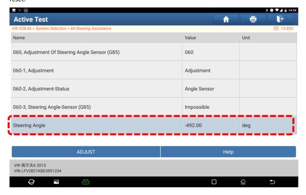
10. When the steering wheel is back to the original direction, the steering angle sensor (G85) must be displayed the value 'Possible', then leave the steering wheel with both hands and click the 'ADJUST' option in the lower left corner.
