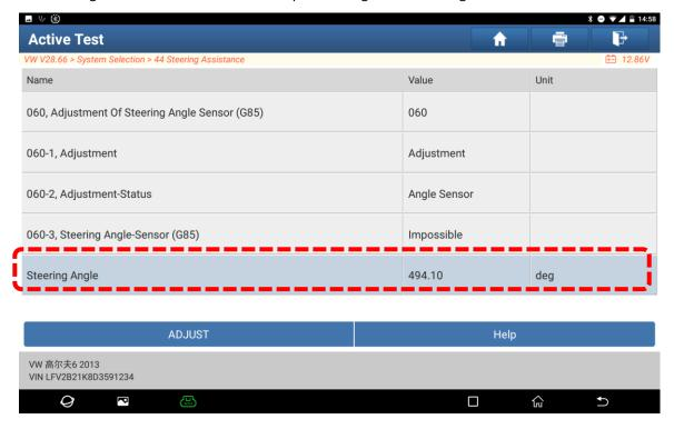
9. The negative angle is 492.00, and the angle difference is within 10 degrees, which can be reset.
