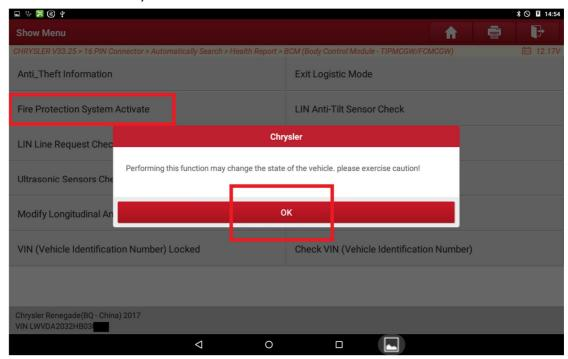
5. This Routine is for use when FPS(Fire Protection System) was activated(If activated blocks the fuel flow). This procedure must be run to re-enable vehicle functionality.
