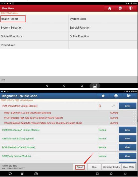
Also, after scanning, we can generate a Report, and share with the technician to assist in analyzing the cause of the failure. It also shows our professionalism and provides a pre-repair vehicle report to customer, for a comparison after the fault is resolved. This is maintenance standard steps and has a very good effect on the analysis of maintenance failures.
