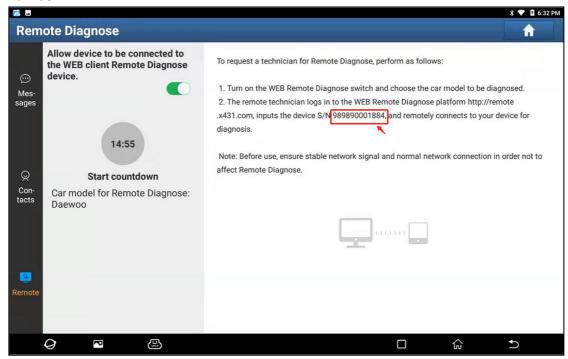
Experienced technicians can log in to remote.x431.com and input the serial number to carry out a remote control on your device.
