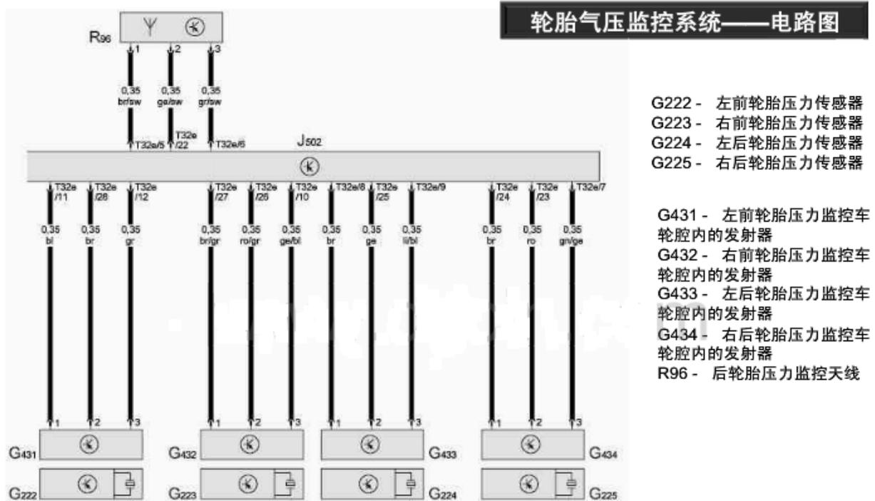
Figure 6 Audi Q7 (China) tire pressure monitoring system
