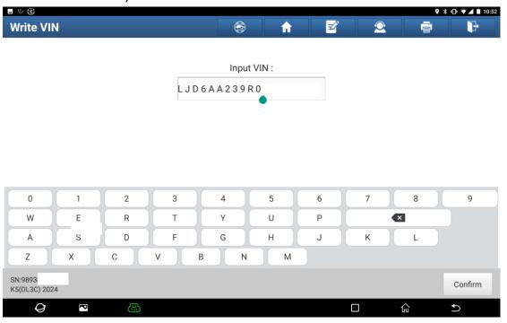
5. Confirm whether the input is correct, and press OK to write.
