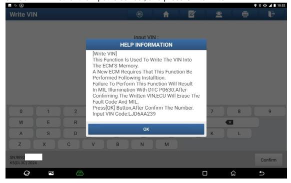
6. After writing is completed, exit the system, turn off the ignition key, and wait for 10 seconds before turning it on again. Then, enter the engine system and use the [Read VIN] function to check whether the writing is successful.
