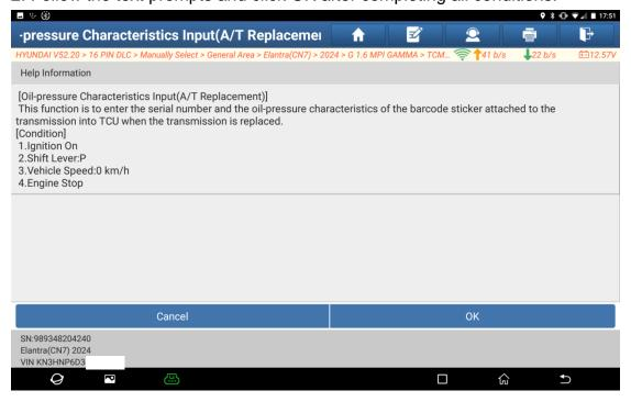
3. Input the serial number and oil pressure characteristics on the barcode sticker attached to the new transmission in sequence, and pay attention to the length and order of each input box to determine the corresponding input data.
