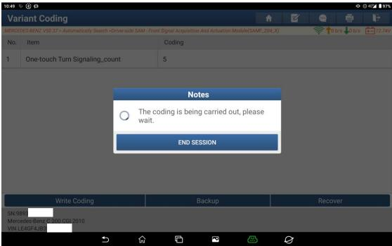
9. The modification is completed. Click OK. Now, when the turn signal stalk is lightly toggled, the turn signals blink for 5 times.
